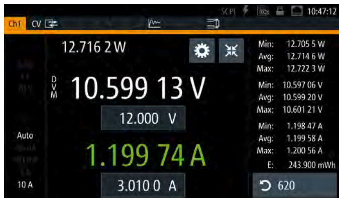
DVM display on an R&S®NGM200 power supply.
